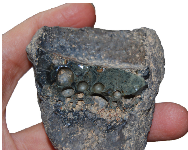
Crucible slag adhering to the interior of a crucible sherd. Credit: Rahil Alipour, UCL
