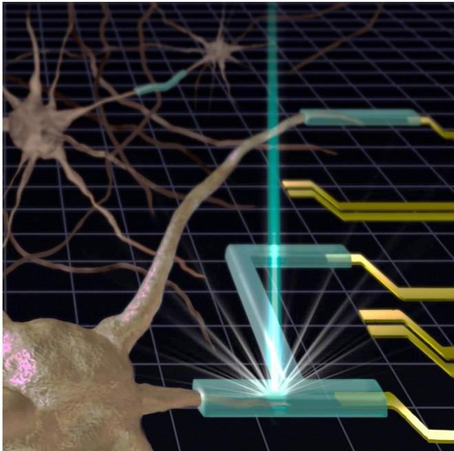
Illustration of a prospective biocompatible interface shows that hydrogels (green tubing), which can be generated by an electron or X-ray beam 3D-printing process, act as artificial synapses or junctions, connecting neurons (brown) to electrodes (yellow). Credit: A. Strelcov/NIST
