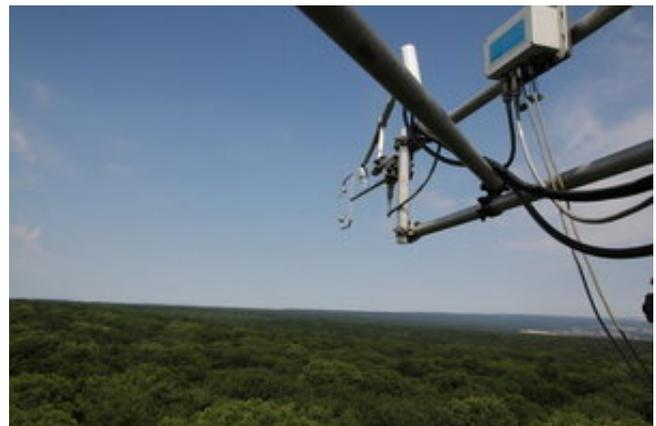
The carbon dioxide and water vapour exchange between forest and atmosphere has been continuously measured at the measuring tower every 30 minutes for 20 years. Credit: Alexander Knohl
