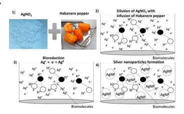
Schematic of the silver nanoparticles' formation by the biosynthesis method. Credit: SPIE
