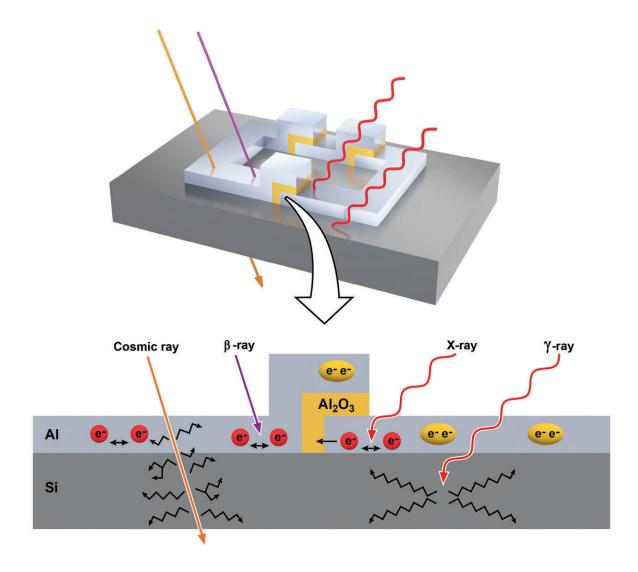
Natural radiation in the form of X-rays, beta rays, cosmic rays and gamma rays can penetrate a superconducting qubit and interfere with quantum coherence. Credit: Michael Perkins, PNNL
