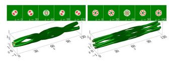
Azimuthon transition between dipole and hexapole, from Zhang et al, doi 10.1117/1.AP.2.4.046002. Credit: Zhang et al.
