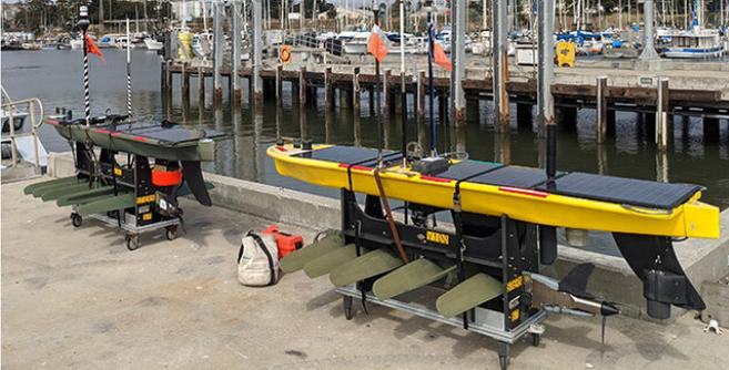
During the Summer 2020 CANON experiment, these two Wave Gliders have been zig-zagging over Monterey Canyon, using echosounders to locate fish and other animals in the water below. The echosounders are the cylindrical devices near the back of each Wave Glider. The olive-green foils under the Wave Gliders help propel these autonomous robots across the sea surface. Credit: Chris Wahl/MBARI
