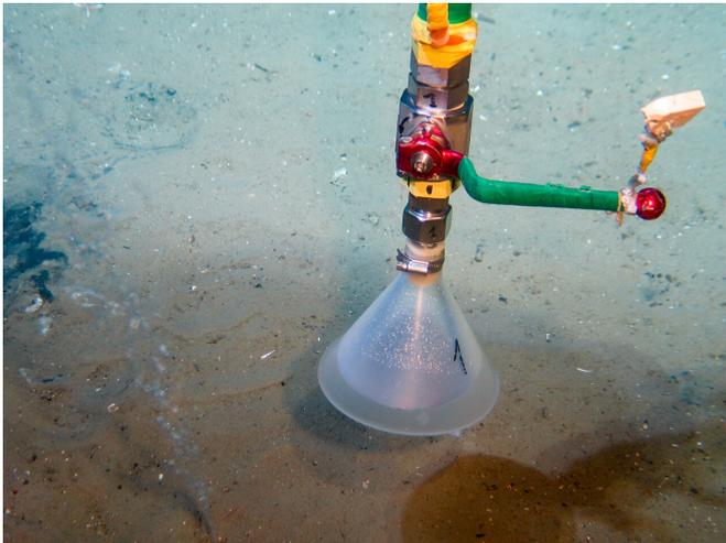
On the basis of investigations directly on the seafloor it was possible to determine the amount of escaping gas. Credit: ROV team/GEOMAR
