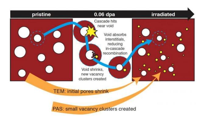
A combination of positron annihilation spectroscopy and transmission electron microscopy reveals new insights into how damage is formed in irradiated materials, suggesting a mechanism in which large holes in the material absorb atoms in interstitial positions in the lattice and shrink, but leave behind more positions that are missing atoms. Credit: Los Alamos National Laboratory.
