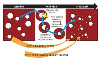
A combination of positron annihilation spectroscopy and transmission electron microscopy reveals new insights into how damage is formed in irradiated materials, suggesting a mechanism in which large holes in the material absorb atoms in interstitial positions in the lattice and shrink, but leave behind more positions that are missing atoms. Credit: Los Alamos National Laboratory.
