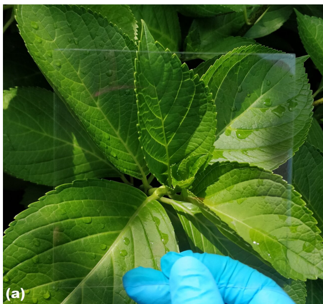
Fig. The samples of transparent EMI shielding materials fabricated through (a) a laboratory facility and (b) a pilot plant facility. Credit: NIMTE
