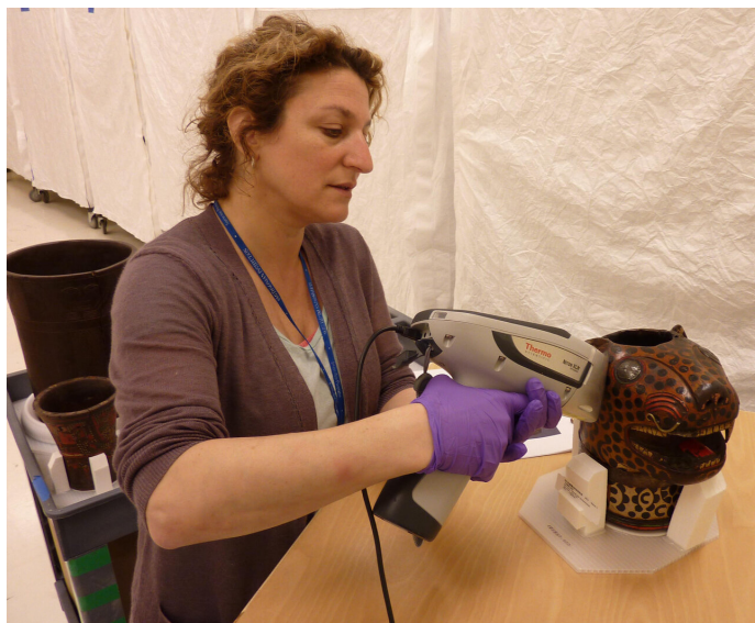
Emily Kaplan using portable X-Ray Fluorescence to detect elements in pigments on a qero at the Smithsonian National Museum of the American Indian. Credit: NMAI staff
