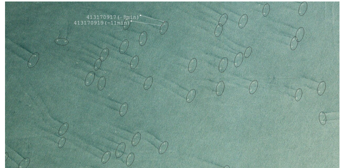
A satellite image of pair trawlers in North Korean waters. Grey ovals show where the neural net classifier identified pair trawlers. In this area, Global Fishing Watch received AIS messages from several vessels (only two shown). White lines connect their most recent AIS position to the estimated position during the time of the satellite image, based on extrapolating the vessel's speed and course. In white is the 9-digit Maritime Mobile Service Identity (MMSI) of each vessel. Credit: © Planet
