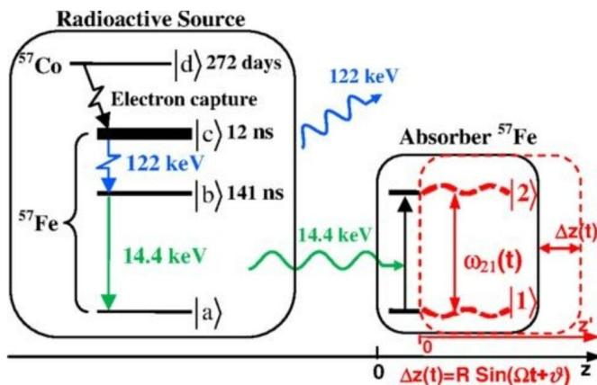
Energy scheme of the radioactive source of 14.4 keV photons and the vibrating absorber used in the experiment. Credit: Kazan Federal University
