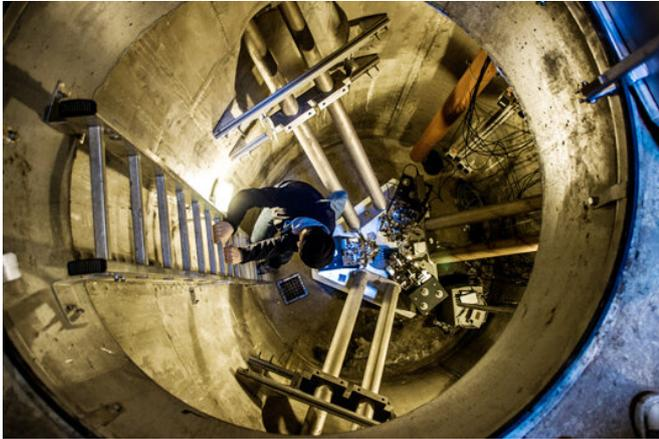
View of the ring laser in Fürstenfeldbruck west of Munich, which can monitor Earth's rate of rotation with high accuracy. It has now determined these parameters with unprecedented precision for a standalone ground-based instrument. Credit: LMU Geophysical Observatory
