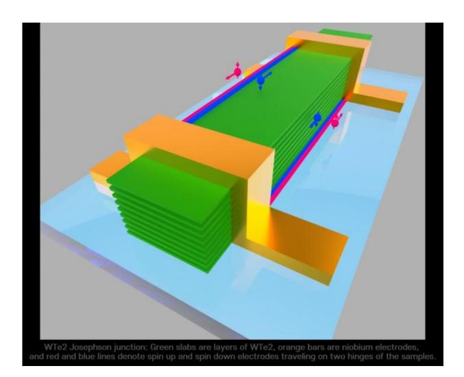
WTe2 Josephson junction: Green slabs are layers of WTe2, orange bars are niobium electrodes, and red and blue lines denote spin up and spin down electrodes traveling on two hinges of the samples. Credit: Gil-Ho Lee (POSTECH)
