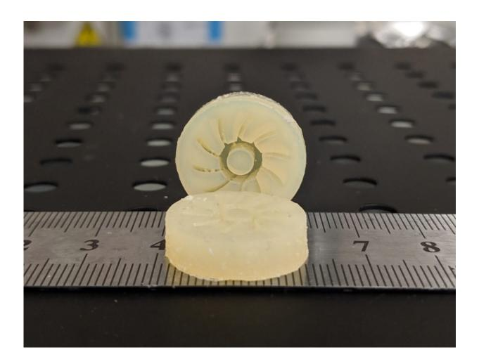
An interdisciplinary group of chemistry and mechanical engineering researchers developed a novel process to 3D print latex rubber. Latex rubber parts, such as this impeller printed at 100 micron resolution, allow nondestructive reuse of complex molds because the parts exhibit a unique combination of flexibility and toughness. Credit: Virginia Tech
