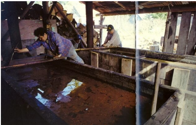
Large vats like the one above are used to cook eulachon and render the valuable oil, or grease. Credit: Kevin Amboe
