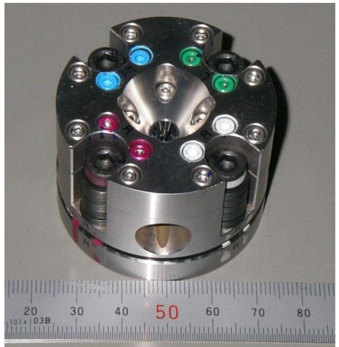
A metal sample is placed inside a rhenium gasket with thermal insulators, squeezed between two diamonds to
