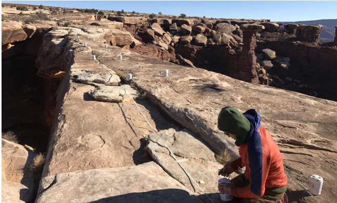
Nate Richman, field assistant, sets up a nodal seismometer. Credit: Paul Geimer.
