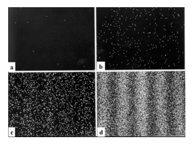
Result of a Young interference experiment: the pattern is formed bit by bit with the arrival of electrons (8 electrons on photo a, 270 electrons on photo b, 2,000 on photo c, and 60,000 on photo d) that eventually form vertical fringes called interference fringes. Credit: <a href="https://doi.org/10.2007/journal/wikimedia">Dr. Tonomura/Wikimedia</a>, <a href="https://doi.org/10.2007/journal/wikimedia">CC BY-SA</a>
