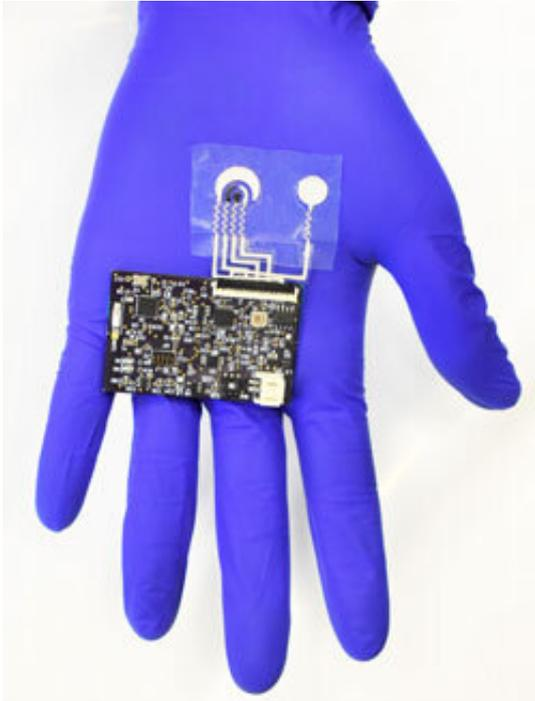
The sensor is paired with a board that can transmit data wirelessly. Credit: University of California - San Diego
