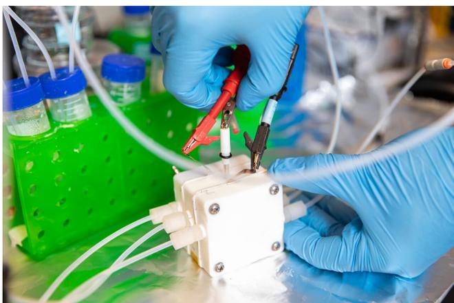
Researchers from U of T Engineering and Carnegie Mellon University are using electrolyzers like this one to convert waste CO<sub>2</sub> into commercially valuable chemicals. Their latest catalyst, designed in part through the use of AI, is the most efficient in its class. Credit: Daria Perevezentsev / University of Toronto Engineering
