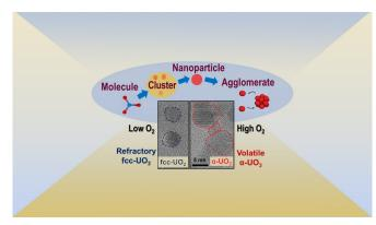
Uranium can prefer to be in metastable oxidation states (i.e., ?-UO<sub>3</sub>) that have higher vapor pressures than refractory forms (i.e., UO<sub>2</sub>) depending on the oxygen abundance in the surrounding environment and rapidity of the vapor condensation process. Credit: Lawrence Livermore National Laboratory
