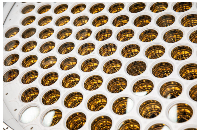
Photomultiplier tube arrays are prepared for the WIMP-hunting LUX-ZEPLIN experiment during assembly at the Sanford Underground Research Facility in Lead, South Dakota. Credit: Matt Kapust/SURF
