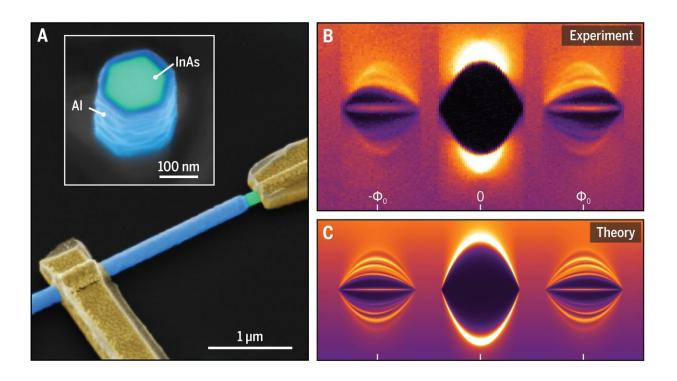
Hybrid material nanowires with pencil-like cross section (A) at low temperatures and finite magnetic field display zero-energy peaks (B) consistent with topological superconductivity as verified by numerical simulations (C). Credit: Nbi
