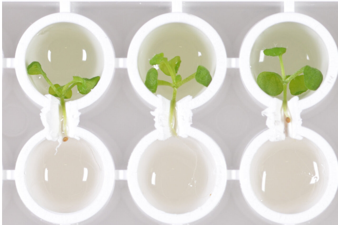
Detail of a modified 96-well plate used by the CRAG researches to simultaneously examine circadian rhythms in the shoot (upper well) and in the root (lower well) of Arabidopsis seedlings. Credit: CRAG
