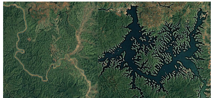
Nai 3, 180 MW hydropower plant, Vietnam. One of a series of 5 hydropower dams built along Nai river in the Cat Tien National Park and UNESCO biosphere reserve. The pictures are from 1996 and 2017 from left to right. Credit: Google Earth
