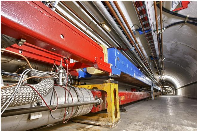
Accelerator magnets can be as long as a pickup truck — sometimes longer — and can weigh tons. It usually takes months to construct each one. They bend and focus particle beams, correct imperfect focusing and even increase beam stability. Credit: Reidar Hahn, Fermilab
