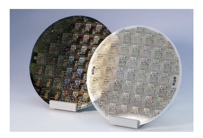
Processed surface acoustic wave (SAW) structures on AlScN/Si layers (left) and AlScN/Al2O3 layers (right). Credit: Fraunhofer-Gesellschaft
