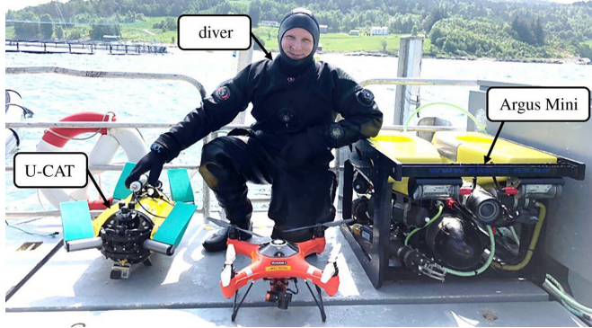
Mobile camera (GoPro3) platforms: the flipper-propelled U-CAT robot (left), human diver and the thruster-driven Argus Mini ROV (right). Credit: Royal Society Open Science (2020). DOI: 10.1098/rsos.191220
