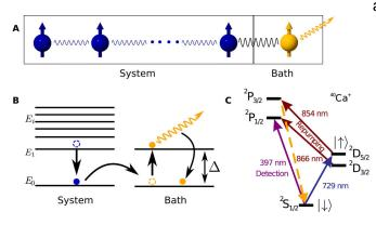
Sympathetic cooling of a quantum simulator. (A) A system of N spins performing the quantum simulation is interacting with an additional bath spin that is dissipatively driven. (B) Sketch of the energy level structure showing resonant energy transport between the system and the bath, after which the bath spin is dissipatively pumped into its ground state. (C) Level scheme for the implementation with trapped 40Ca+ ions. Credit: Science Advances, doi: 10.1126/sciadv.aaw9268
