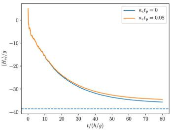
Cooling performance of an Ising-like chain of 5 + 1 ions of tp = 80?/g = 24s. The blue line shows the dynamics in the decoherence-free case resulting in a fidelity of f = 0.92, while the orange line indicates the dynamics under a collective decoherence mechanism with rate ?c = 3.3Hz, resulting in f = 0.89. The dashed line indicates the ground-state energy of the system. Credit: Science Advances, doi: 10.1126/sciady.aaw9268
