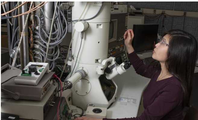
NIST researcher June Lau with a transmission electron microscope (TEM) that she and her colleagues retrofitted in order to make high-quality atom-scale movies. Credit: N. Hanacek/NIST
