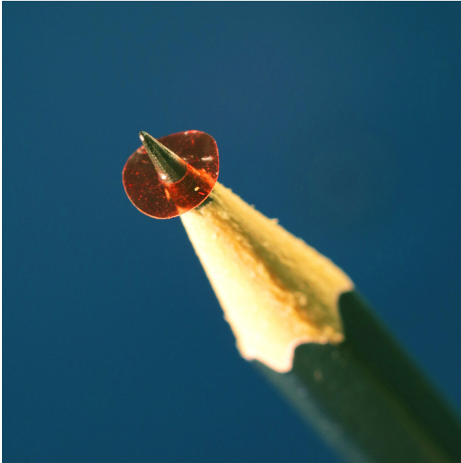
Photo of the 5.5 mm diameter micromotor rotor made of specially oriented polymer film, on a pencil tip. Credit: UW Physics, Piotr Wasylczyk
