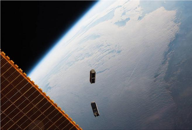
Two CubeSats, part of a constellation built and operated by Planet Labs Inc. to take images of Earth, were launched from the International Space Station on May 17, 2016. Credit: [NASA](#)
