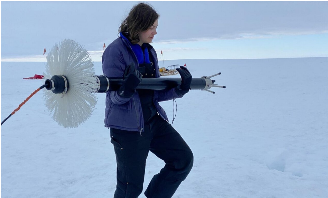
NYU graduate student Aurora Basinski carries a turbulence measuring device to the borehole on Thwaites Glacier. Credit: David Holland, NYU and NYU Abu Dhabi
