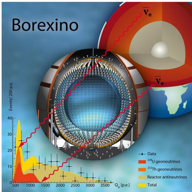
The diagram shows geoneutrinos from the earth's interior measured by the Borexino detector, resulting in the final energy spectra. The x-axis shows the charge (number of photo electrons) of the signal, which is a measure of energy deposited in the detector, and the y-axis shows the number of measured events. Credit: Borexino Collaboration
