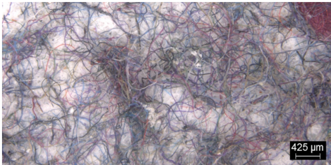
Microscopic microfibrils filtered from the test washing loads. Credit: University of Leeds/P&G
