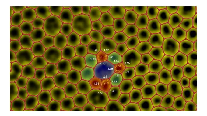
Researchers at NUS have created the world's first atomically thin amorphous carbon film. The amorphous structure have widely varying atom-to-atom distance unlike crystals. This is because of the random arrangement of five-, six-, seven- and eight-carbon rings in a planar carbon network, leading to a wide distribution of bond lengths (in Å) and bond angles. Credit: National University of Singapore
