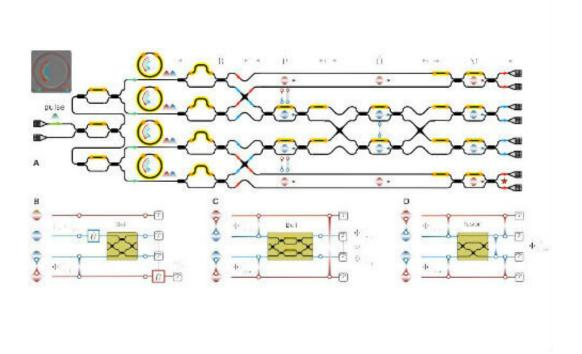
A. Chip Schematic. Black lines represent single mode waveguides for the single photons, red and blue pulses represent the photon energy in each path. Yellow bars represent external phase control. B. Teleportation setup. C. Entanglement swapping setup. D. 4-photon GHZ state preparation. Credit: University of Bristol
