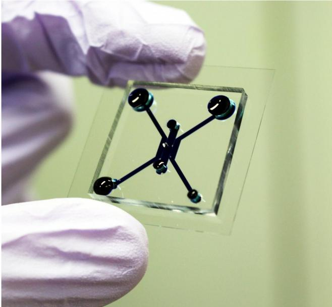
The device allows researchers to mimic the environment inside the body to screen for better cancer screening drugs. Credit: Kyoto University/Yokokawa Lab
