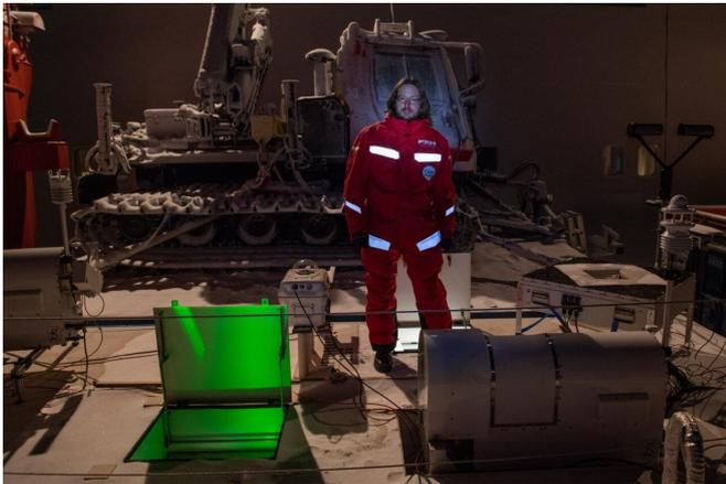
Dr. Ronny Engelmann from TROPOS supervises the lidar measurements in the OCEANET container on the foredeck of Polarstern during the first section of the MOSAiC expedition. From the lidar only the green scattered light can be seen in the roof hatch. The laser beam itself cannot be seen because of the relatively clean air on the ground. Credit: Alfred-Wegener-Institut / Esther Horvath (CC-BY 4.0)
