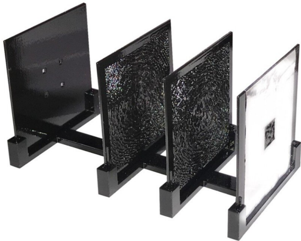
Prototype of a broadband diffractive deep neural network. Credit: Ozcan Lab @ UCLA
