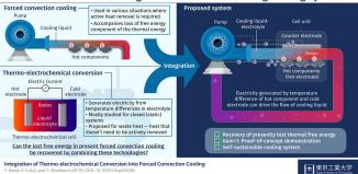
Schematic illustration of the concept on the integration of thermo-electrochemical conversion with forced convection cooling to create a self-sustaining cooling system. Credit: Tokyo Tech
