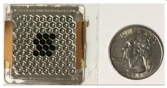
A new solar power generator prototype developed by Ben-Gurion University of the Negev (BGU) and research teams in the United States, will be deployed on the first 2020 NASA flight launch to the International Space Station. The first prototype pictured here holds 90 miniaturized solar concentrators, and shows 12 solar cells with the concentrators in black. Credit: Ben-Gurion U./Jeffery Gordon
