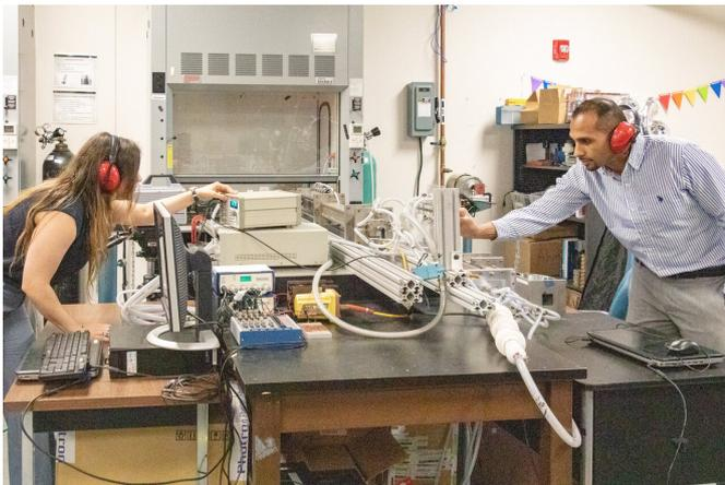
Jessica Chambers, a doctoral student in the University of Central Florida's Department of Mechanical and Aerospace Engineering, and Kareem Ahmed, an assistant professor in UCF's Department of Mechanical and Aerospace Engineering, set up the turbulent shock tube they used to help uncover the mechanisms that could have caused the Big Bang. Credit: Karen Norum, UCF Office of Research
