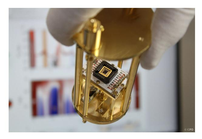
Close-up of the device placed onto the piece that later is adjusted to the experimental setup ©ICFO Credit: ICFO
