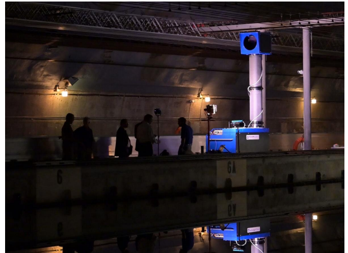
A two-kilowatt laser transmitter atop a 13-foot-high tower, part of the long-range, free-space power beaming system. Credit: Leonard Pieton
