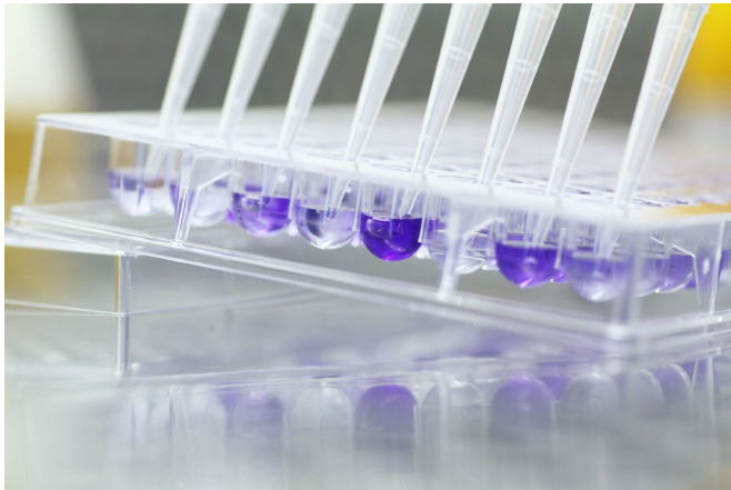
Close-up of a so-called diagnostic Biolog plate, with which the metabolic activity of bacteria is measured. Credit: Christian Urban, Kiel University
