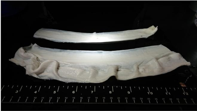
Gelatin fibers produced by 'immersion rotary jet spinning', a fiber production system inspired by cotton candy. These fibers form the 'base' to grow cells in -- they mimic natural muscle tissue's extracellular 'glue', which holds the tissue together and contribute to its texture. Credit: Harvard University
