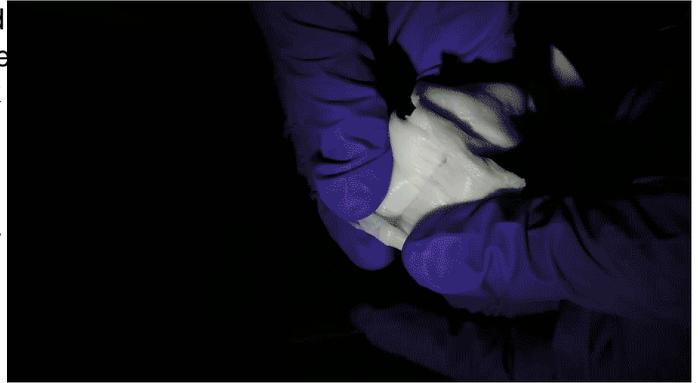
Peeling apart gelatin fibers produced by immersion rotary jet spinning. These fibers mimic long, thin muscle fibers. Credit: Harvard University
