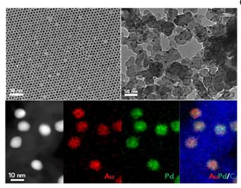
A new catalyst made from alloyed nanoparticles of gold and palladium can produce PBO polymer, which is used in body armor and other high-performance fabrics. The new catalyst produces PBO that's free of impurities, which can cause materials to degrade. Credit: Sun lab / Brown University
